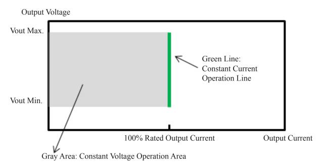
Note: The Constant Current LED driver is designed to work in the constant current mode (on the green line above). Depending on the LED loads connected to the driver, it can output the regulated rated current with a voltage sitting in between the Vout max and Vout min. However, the driver will switch to constant voltage mode if the current draw from the LED loads is lower than the rated current of the driver. Please contact Amperor for detailed explanations.
